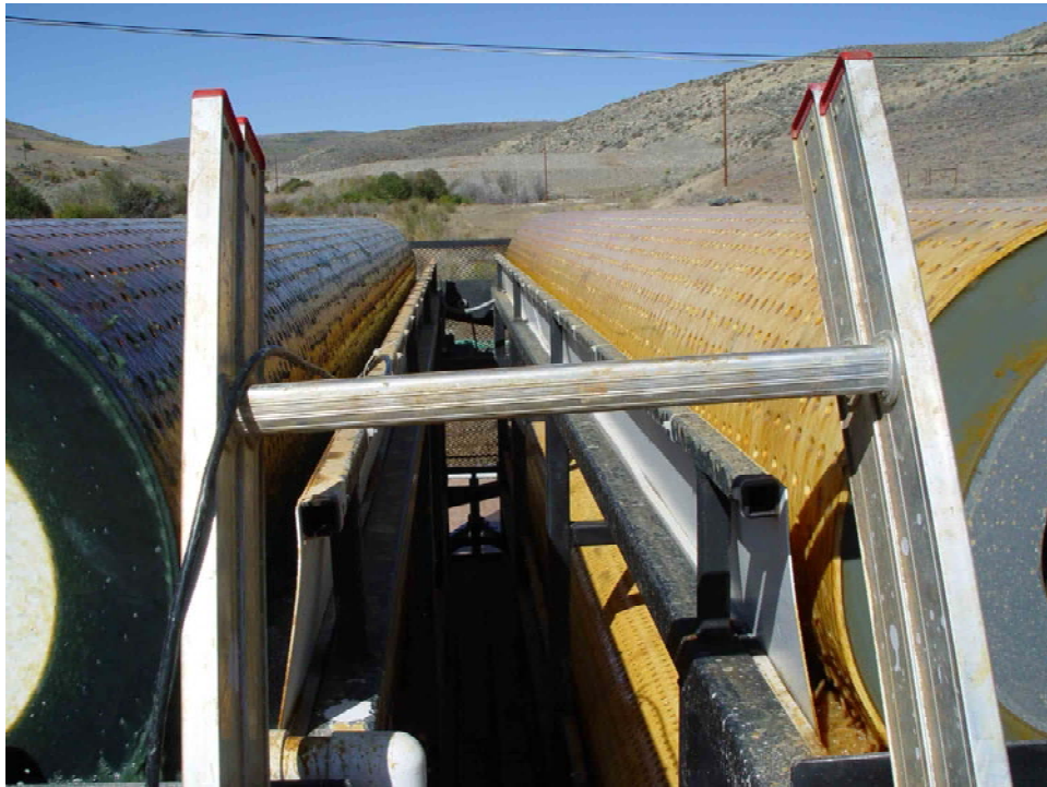
Figure 2. Iron oxidation from ferrous to ferric in the first two cylinders of the four rotor unit.
